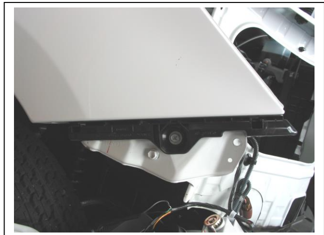
Figure 6 - Remove plastic bumper support from under guard.
