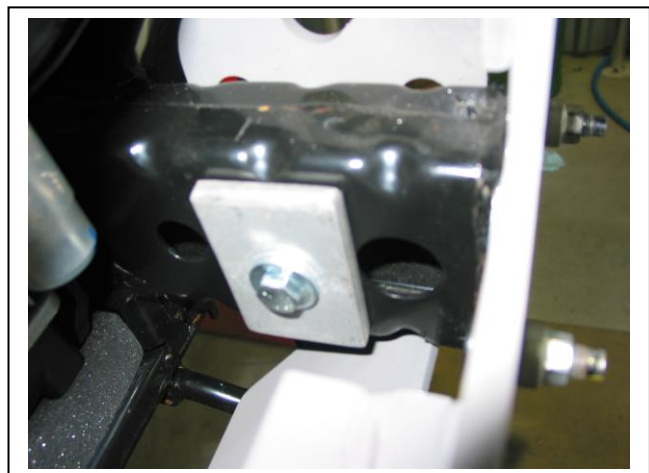
Figure 6 – Washer straight to vehicle
