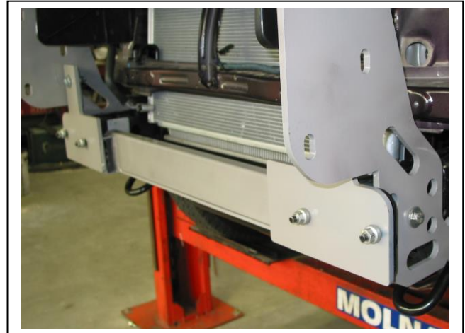
Figure 8 – ECB steel mounting brackets fitted
