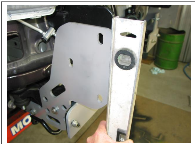
Figure 9 - Passenger side shown Levelling off front edge
